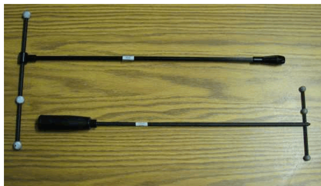
Figure 7. 240 mm and 120 mm camera calibration wands. Each has three reflective markers.
